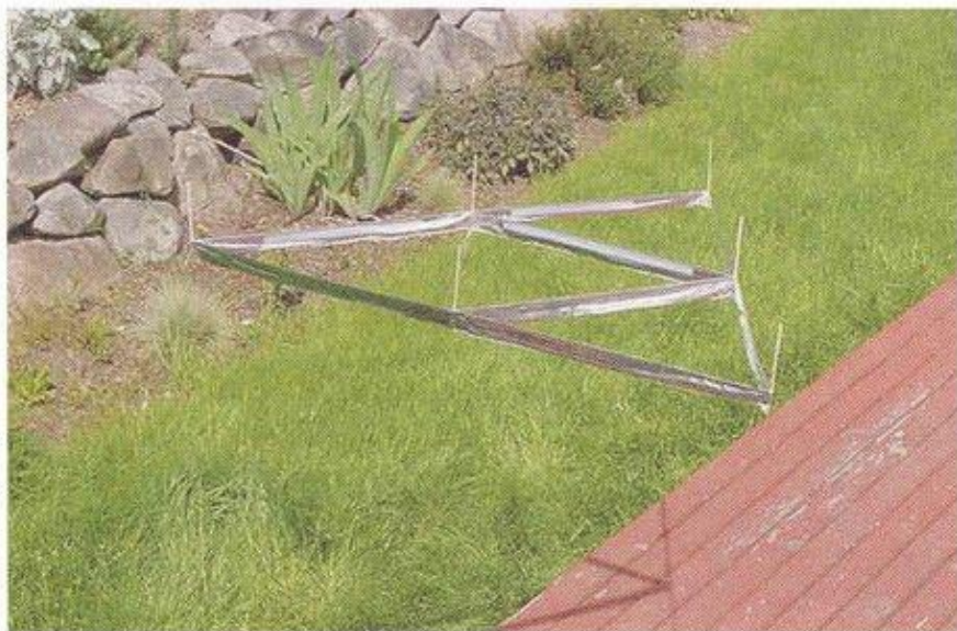
GETTING THINGS OFF THE GROUND: The Lifter, while not a 'true' antigravity device, produces directional thrust using an electromagnetic propulsion system that has no moving parts.
